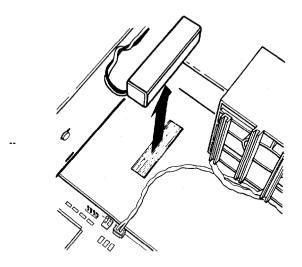
3. Remove the new battery from its package and position it so the Velcro faces down and the cable faces connector CN1. Then attach it to the bottom of the computer case, as shown below.
